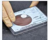
FIRMLY RESEAL InTray by pressing the edges of the label and the plastic tray together. Complete the label with patient information in accordance with your laboratory requirements.
