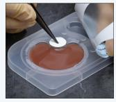
Before incubation, puncture the seal over the  ${\rm CO}_2$  Chamber with the pointed objected.
