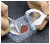
Allow the InTray to warm to 18-25°C (64-77°F)! Manually pull the lower right corner (adjacent to the clear window) back so that the protective seal is completely visible.
